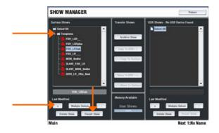
Note: Recalling a Show overwrites all the system settings including the DSP mix architecture, Surface configuration, current parameters, all the Scene and Library memories. If you want to keep the current configuration make sure you archive it as a User Show before recalling the new Show.
